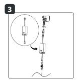
Now connect the coupling piece of the strip to the coupling piece of the strip dimmer and connect the coupling piece of the strip dimmer to the product cable connector.
