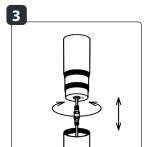
Connect the wiring of the housing to that of the lamp, then screw the housing onto the lamp.
