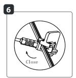
Attach the product connector to the 12-volt main cable and tighten the connector onto the main cable. Your lighting is now ready for use.
