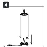
Option 1: Detach the bottom by unscrewing the 3 hex screws using the included hex key. Then, mount the bottom with the 3 provided screws at the desired position. Afterward, screw the top back onto the mounted bottom and secure it with the 3 hex screws.
