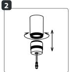
Tighten the lamp onto the bottom of the casing.
