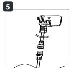
Connect the coupling piece of the standing light to the product cable connector.
