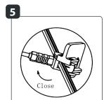
Attach the product connector to the 12-volt main cable and tighten the connector onto the main cable.
