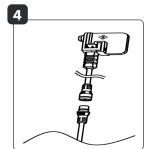
Now connect the coupling piece of the spike light to the product cable connector.
