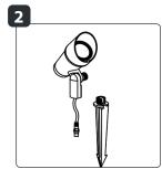
Twist the spike onto the fixture. Note: Place the cable in the notch of the spike.
