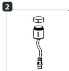
Screw the top onto the ground light.
