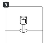
Drill a hole with a diameter of 25 mm at the desired location and insert the ground light into the hole. If necessary, use the supplied strike plate.
