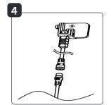
Now, connect the ground light's coupling piece to the product cable connector.
