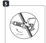
Now insert the 12-volt main cable between the product cable connector and click the connector securely onto the main cable.
