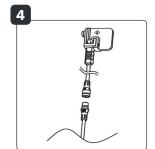
Connect the coupling piece of the wall light (or the 12-volt extension cable) to the product cable connector.
