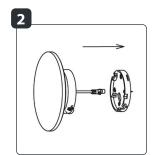
Unscrew the screw located at the top of the wall-mounted fixture and separate the fixture. Attach the fixture to the wall using the 4 included screws. Then, screw the other side of the fixture onto the wall light and connect the wiring coming from the wall to the cable of the wall light.
