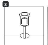
Drill a hole with a diameter of 32 mm at the desired location and insert the ground light into the hole. If necessary, use the supplied strike plate.
