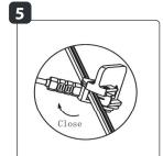
Place the 12-volt main cable between the product cable connector and snap the connector onto the main cable. Your lighting is now ready for use.
