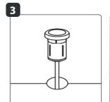
Drill a hole with a diameter of 25 mm at the desired location and insert the ground light into the hole. If necessary, use the supplied strike plate.
