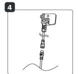
Now, connect the coupling piece of the ground light to the product cable connector.
