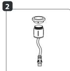
Screw the top onto the ground light.
