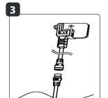
Now, connect the coupling piece of the ground light to the product cable connector.
