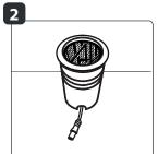
Without the mounting tube: drill a hole with a diameter of 63 mm at the desired location and insert the ground light into the hole.
