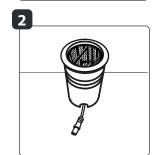
Without the mounting tube: drill a hole with a diameter of 40 mm at the desired location and insert the ground light into the hole.
