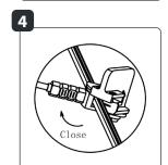
Place the 12-volt main cable between the product cable connector and snap the connector onto the main cable. Your lighting is now ready for use.
