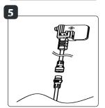
Connect the coupling piece of the wall light (or the 12-volt extension cable) to the product cable connector.
