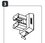
Secure the fixture by tightening the screw at the bottom.
