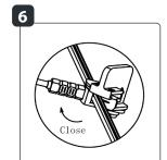
Now insert the 12-volt main cable between the product cable connector and click the connector securely onto the main cable. Your lighting is now ready for use.
