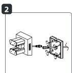
Unscrew the screw located at the bottom of the wall-mounted fixture and separate the fixture. Attach the fixture to the wall using the 4 included screws. Then, reassemble the other side of the fixture onto the part already mounted on the wall.
