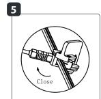
Attach the product connector to the 12-volt main cable and tighten the connector onto the main cable.
