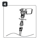
Now, connect the coupling piece of the spike light to the product cable connector.
