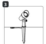
Push the spike into the ground at the desired location.
